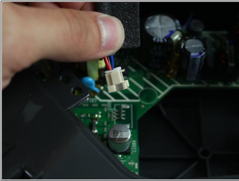
! The motherboard contains capacitors (shown as cylinders in the upper right of the picture) which can hold a charge even when the speaker is powered off. Do not touch them as doing so may result in a shock.
