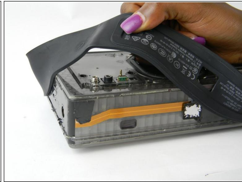
**⚠** Be gentle, the rubber seal is fragile and easy to tear, resulting in cosmetic damage to your device.
