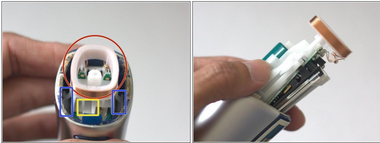
⚠ Do not pull the coil ring as the wire will break away from the the circuit board
