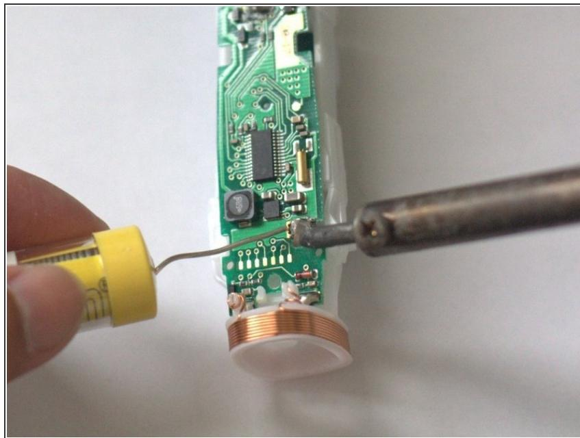
! Make sure you respect the polarity when you are placing the new battery (see step 6)
