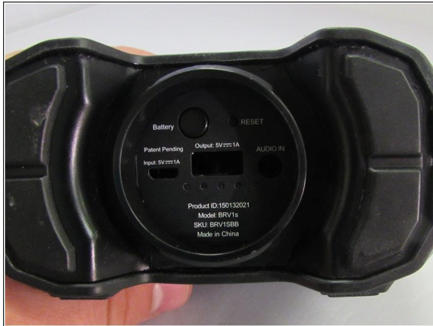
when screwing in the replacement rear water cap, ensure it is properly aligned to ensure the device remains waterproof
