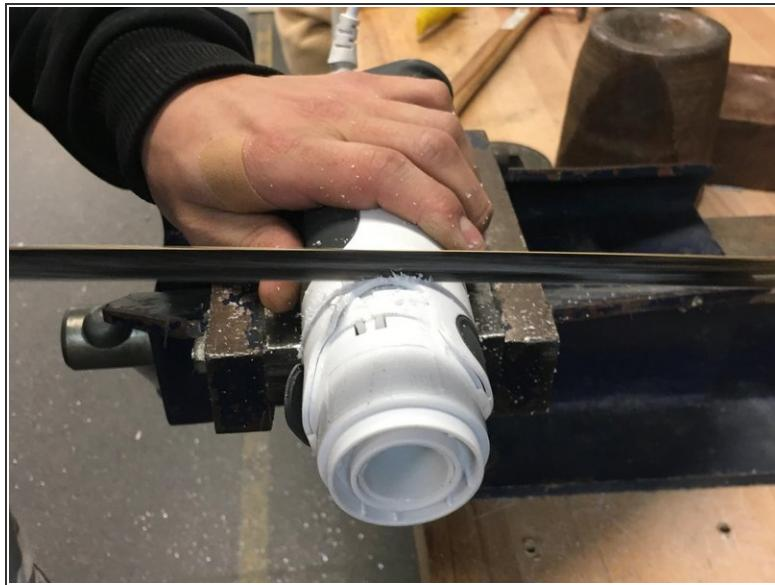
**⚠ This step will damage your product but is the simplest and most effective way to access the motor components/PCB as the case is plastic welded to minimise moving parts when the blender is in use.**
