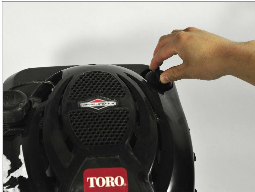
**⚠** Make sure the the engine is off and the spark plug wire is removed and away from the spark plug before beginning.
