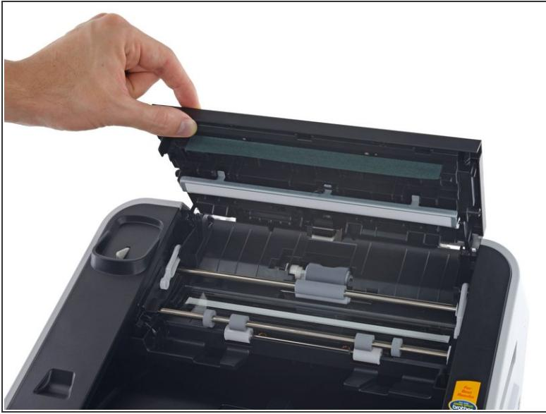
**⚠** Do not attempt to completely remove the control panel yet, as it is still connected by a cable.
