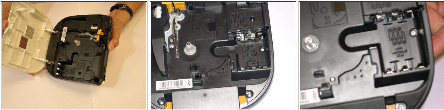
! For safety precautions, it is advised that you remove the batteries before trying to remove and replace your tape cassette.
