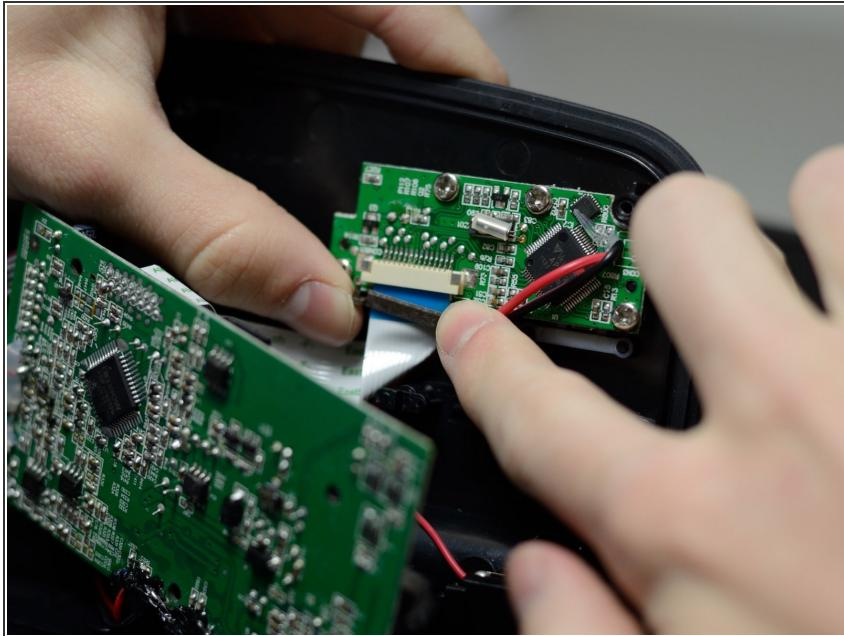
**⚠** There is ribbon wiring under this PCB. Be careful not to damage it while removing the PCB.
