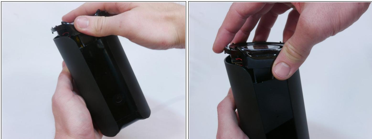
! Do not yank the bottom off or you may damage the ribbon cable or the ZIF connector.
