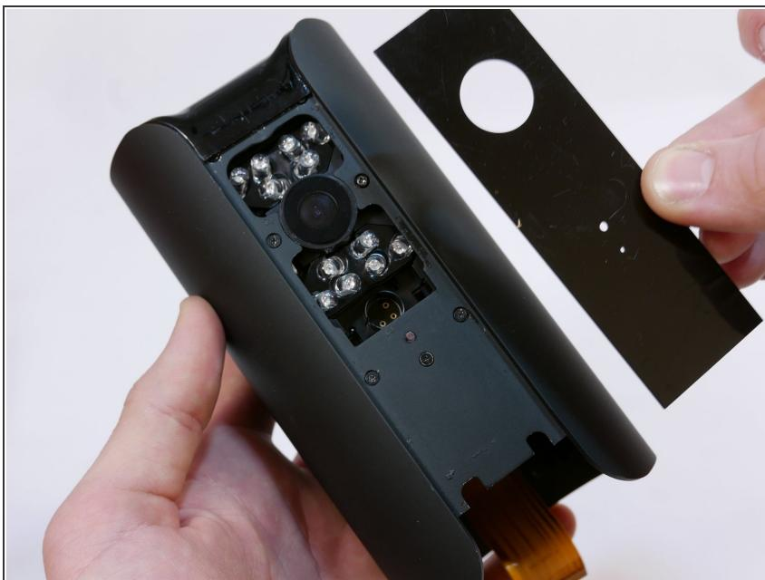
*(i)* Adhesive will have to be reapplied after removing the panel.
