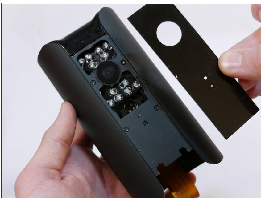
*(i)* Adhesive will have to be reapplied after removing the panel.
