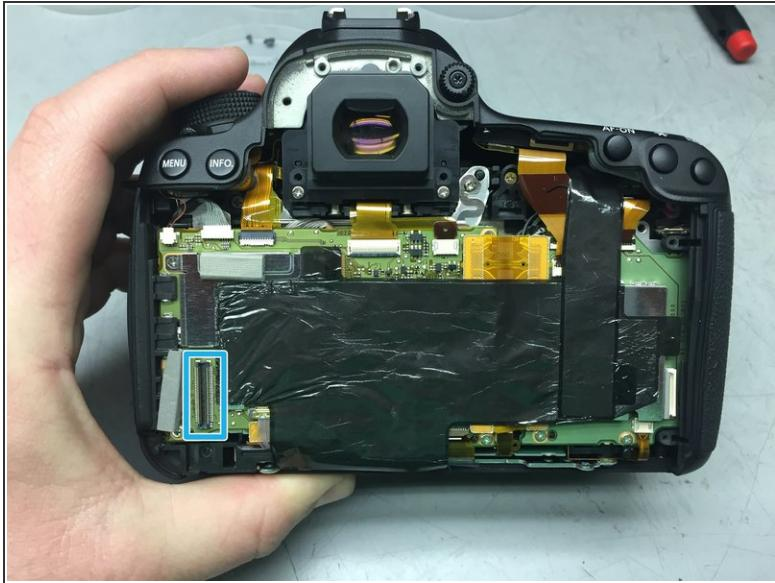
⚠ You can now lift straight up on the back plate and separate it from the body. Be careful to raise it gently because on the left side it is still connected with a ribbon cable to the main pcb.
