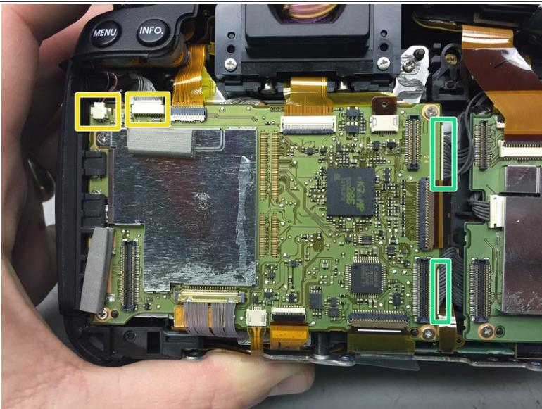
! From this point on, be very careful. We will be removing or dislodging internal connectors that may be damaged if not careful and will impact the camera functions if not seated correctly when put back together.
