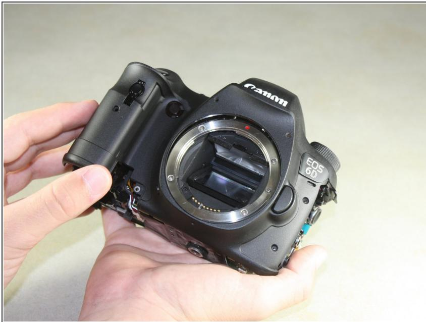
**⚠** The red speaker wire is attached to the inside of the front panel. Opening the front panel forcefully may break it.
