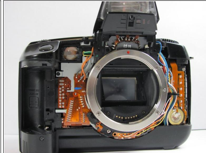
**⚠ Starting at the flash, carefully pull the front cover away from the camera.**
