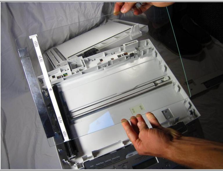
**⚠** After you have taken off the plate, check to make sure that there is no broken glass. If there is broken glass handle it with gloves. Broken glass, if handled improperly, can cause physical injury.
