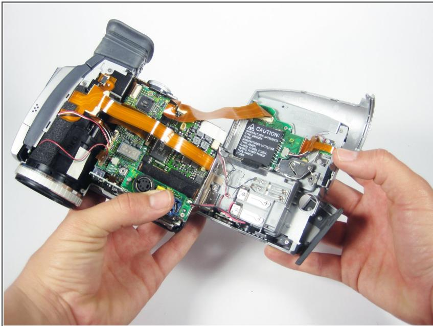
**⚠** The side of the device should now be open as shown. Again, there are wire connections between the side cover and the body of the camcorder. Do not separate the two entirely!
