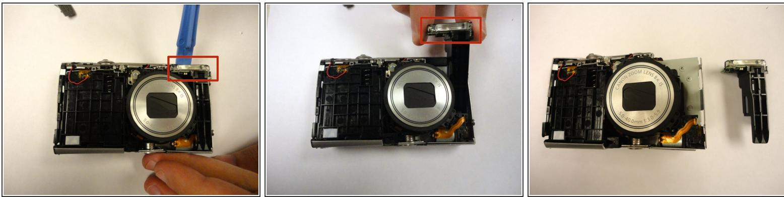
**⚠** The flash is not held very securely in the camera so be careful. Make sure someone is holding onto it so it does not fall out.
