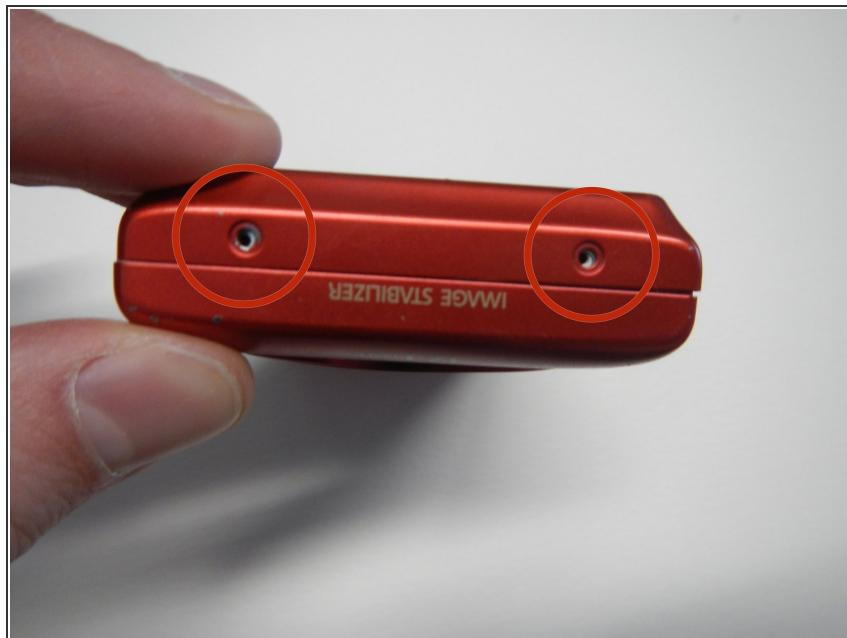
⚠ Be careful when removing screws, as they are stripped easily.
