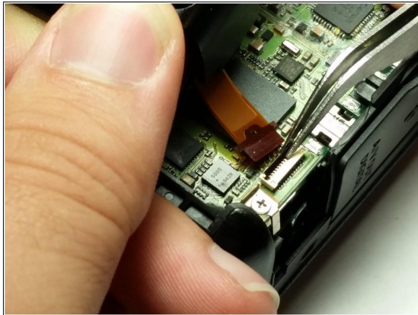
! The rear case is still attached to the camera with a ribbon cable. The socket has a flip up lid that must be flipped up before the cable can be removed. Use the tweezers to flip the cable attachment up.
