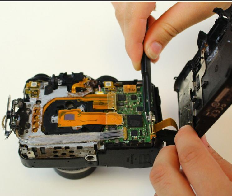
**!** The back case is still attached to the camera with a yellow ribbon cable. The socket has a black flip-up lid that must be flipped up before the cable can be removed. Use precision tweezers to remove the cable.
