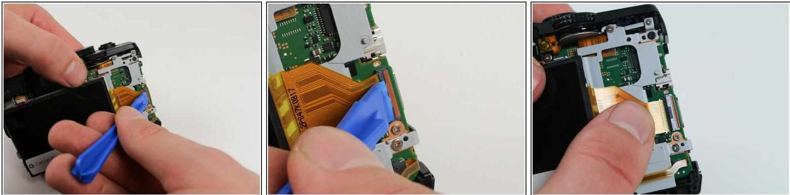
! Do not pull the connector upwards as doing so may harm the connector housing.
