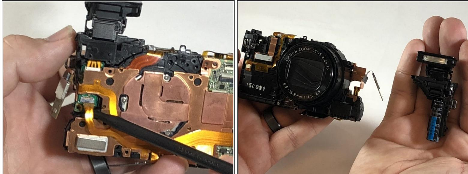
⚠ Flash contains charged capacitor. Shock hazard.
