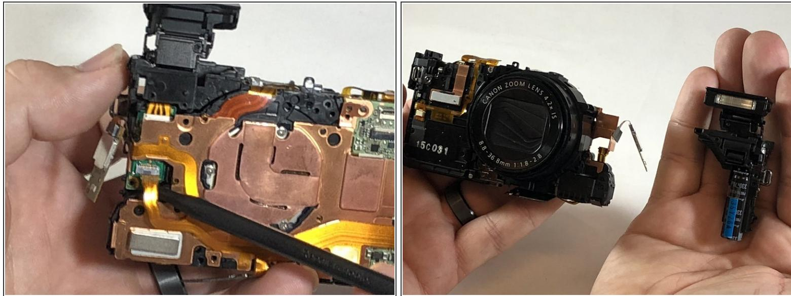
⚠ Flash contains charged capacitor. Shock hazard.
