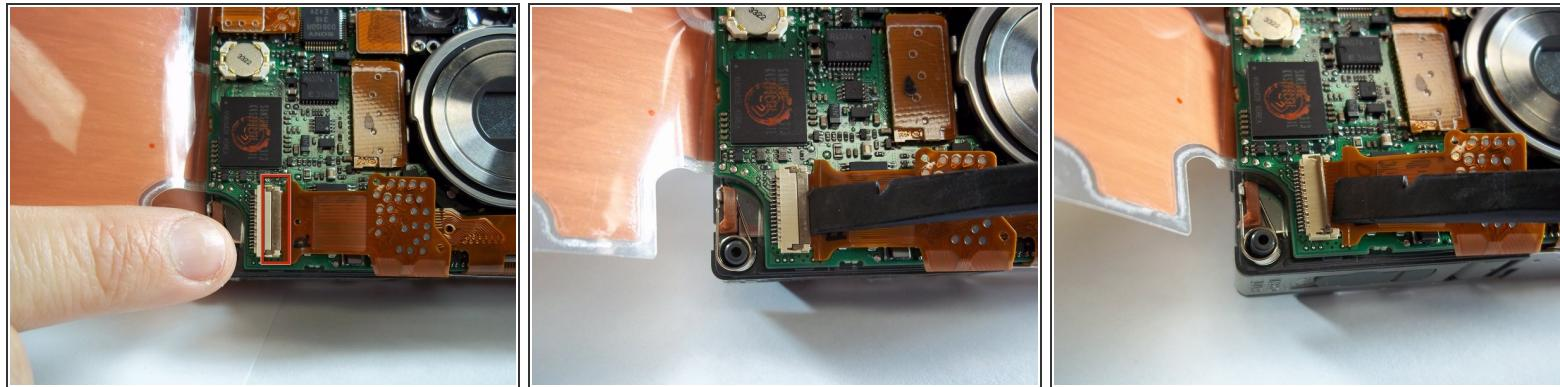
**⚠** The motherboard can be damaged easily and must be treated with care. Try to avoid removing ribbon cables with your fingers, since motherboards are extremely sensitive to static discharge. Use a spudger or plastic opening tool to lift any flaps or tabs or to pry connectors straight off their sockets on the motherboard.
