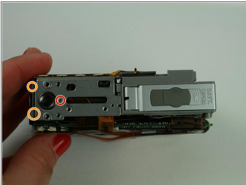
**⚠** Do not remove the metal plate this step refers to. Removal at this step may damage the ribbon cable. Wait until the next step to remove the plate.
