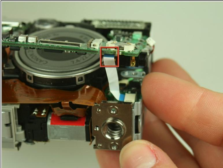
**⚠** Do not completely remove the main circuit board from the camera. A soldered ribbon cable still attaches the board to the camera. Complete removal would break the soldering points.
