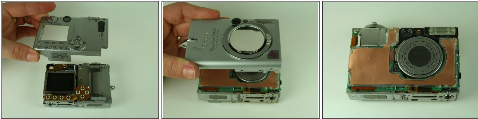
**⚠** There is a small black plastic piece that sits above the lens underneath the camera case. This plastic piece may fall out when you remove the cases; recover the piece and save it.
