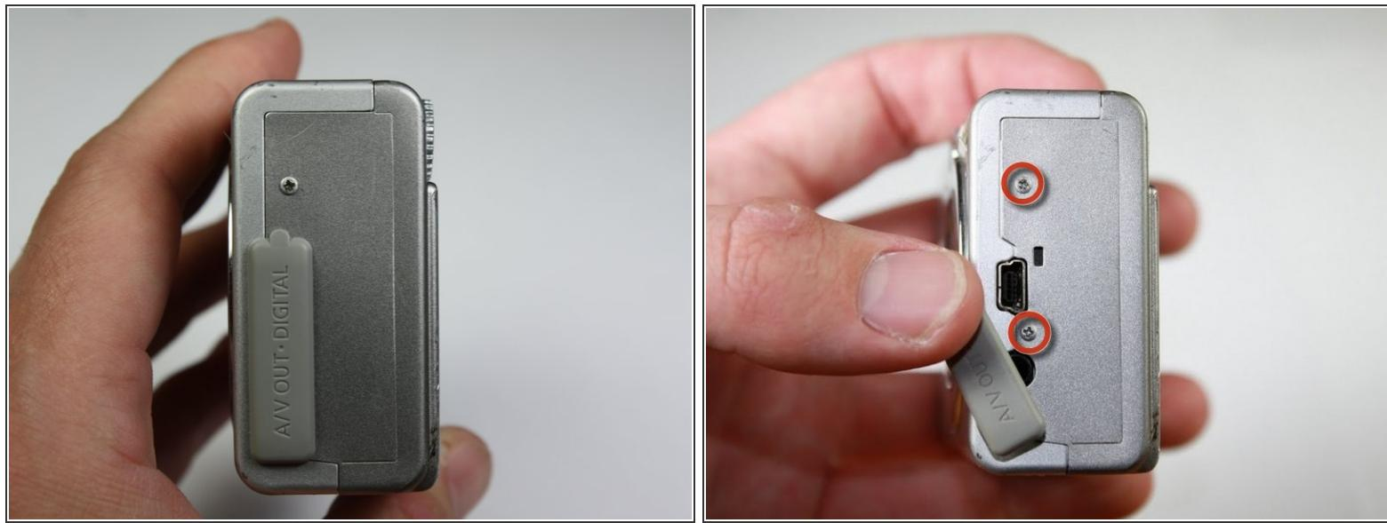
*(i)* Position the camera so that the rubber "AV Out Digital" tab is facing upward.
