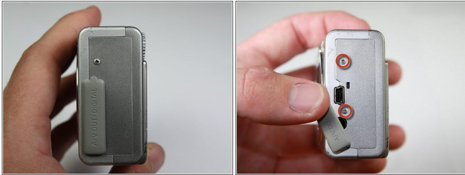
*(i)* Position the camera so that the rubber "AV Out Digital" tab is facing upward.
