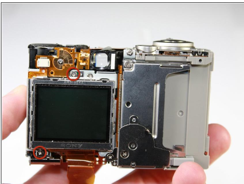
*(i)* Turn the camera so that the LCD screen is facing you.
