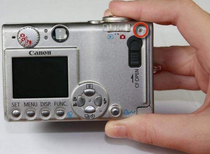
*i* Start by laying the camera flat with the LCD screen facing up.
