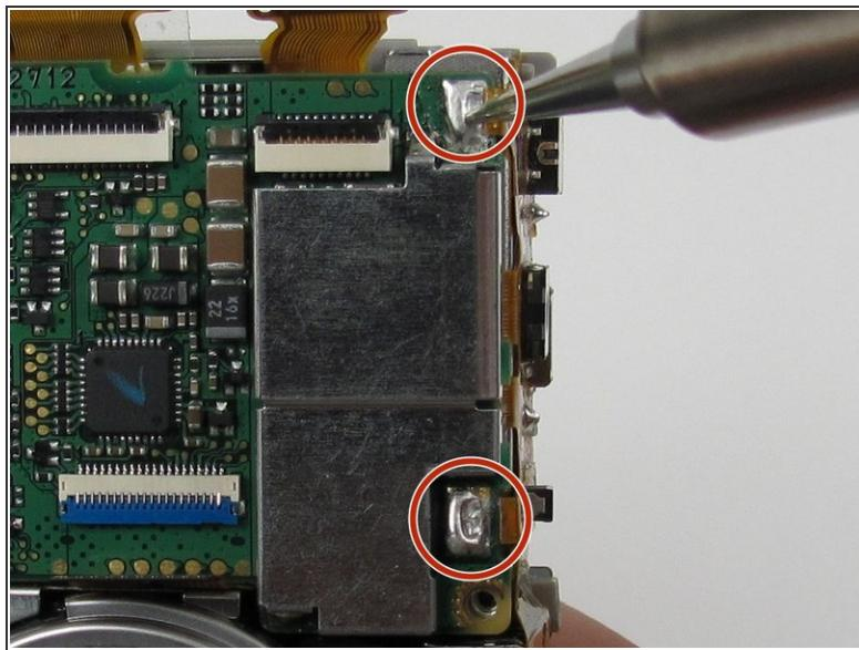
*(i)* We're now ready to begin the desoldering process. You'll need a soldering iron, solder, and desoldering wick. You should be able to find these items at a Radio Shack if you don't already have them.
