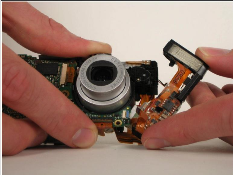
**⚠** Before working on the flash assembly make sure the flash is completely discharged or pay attention to where your fingers are. The capacitor in the flash assembly can hold a charge for a long time and it can shock you.
