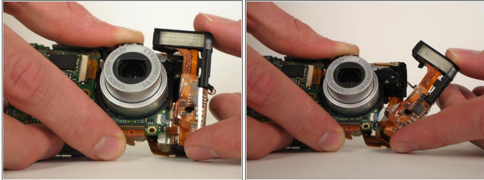
**⚠** Before working on the flash assembly make sure the flash is completely discharged or pay attention to where your fingers are. The capacitor in the flash assembly can hold a charge for a long time and it can shock you.
