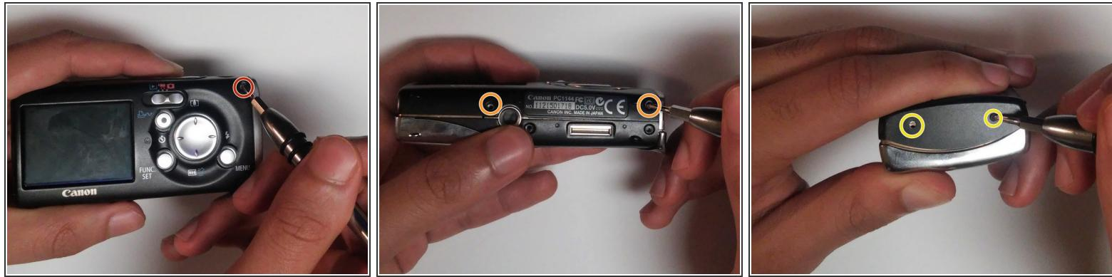
① Remove the wrist strap and battery before removing the back cover.
