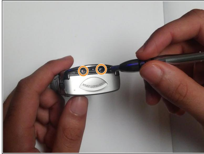
*(i)* Be sure to remove the wrist strap and battery before removing the cover.
