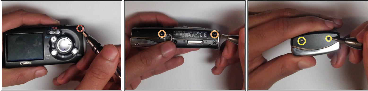
ⓘ Remove the wrist strap and battery before removing the back cover.
