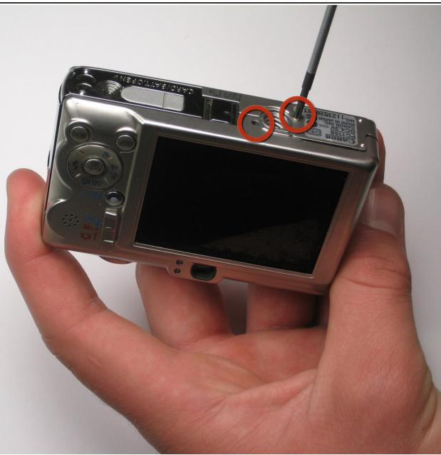
⚠ Remove the battery and SD Card from their slots. Leaving these in could cause the battery to ground and ruin the electronics.
