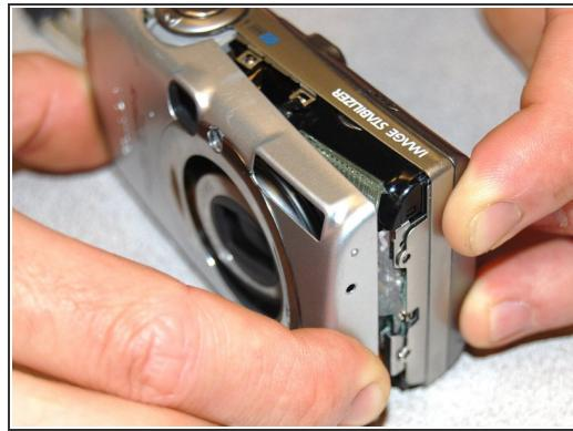
**⚠** To avoid severe electric shock do not remove or tamper with internal camera flash components. An electrical capacitor is attached to the flash that can discharge if contact is made.
