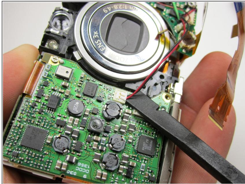
*i* Pay special attention when removing this connector. It does not pull out like the rest of them. Instead, you must use a spudger to lift the connector vertically out of its slot.
