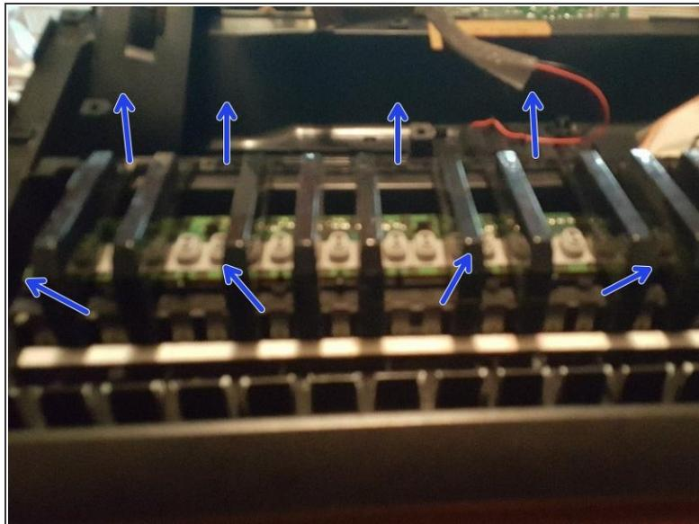
**⚠ Be sure to hold everything together as you turn the keyboard over. Be especially careful of the ribbon cable going to the left-most side of the keyboard.**
