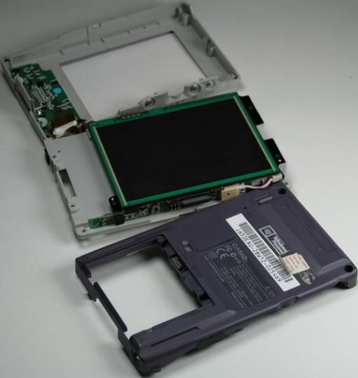
**⚠ Caution:** be careful not to pull out the wires connecting the two halves of the outer case. These wires are necessary for the device to be able to function.
