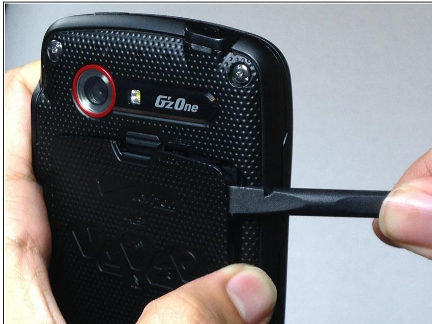
**i** This device is waterproof and well sealed, so it is difficult to open this handset.
