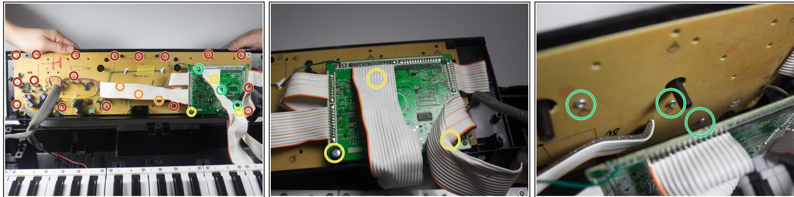
*(i)* In this step, you will be removing a total of 26 screws.
