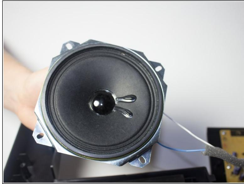
*(i)* A soldering iron is needed to remove the wires connected to the speaker in order to fully replace it. For soldering help, take a look at the [Soldering and Desoldering Connections](#) guide.
