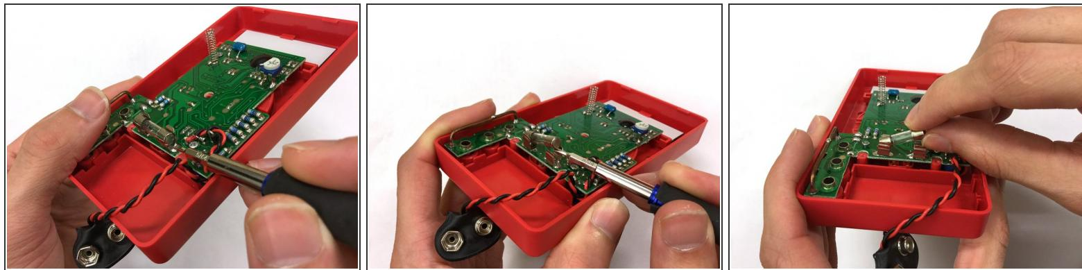
**⚠** Avoid touching any parts of the circuit board. Electronic devices are sensitive to small static shocks. You can get rid of excess static electricity by touching any large and metal, such as a fridge, stove, or metal rack.
