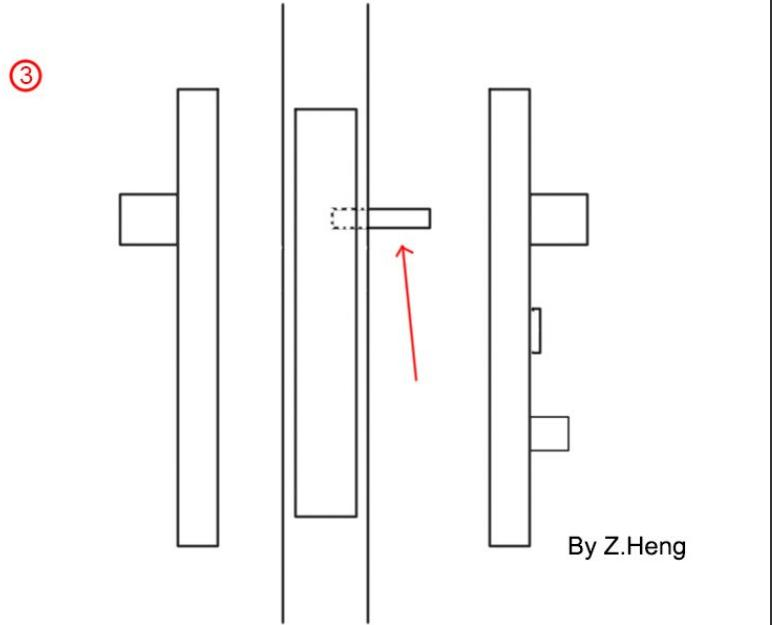
⚠ Pay attention to the installation direction of this square shaft. Do not knock it off when removing the handle.
