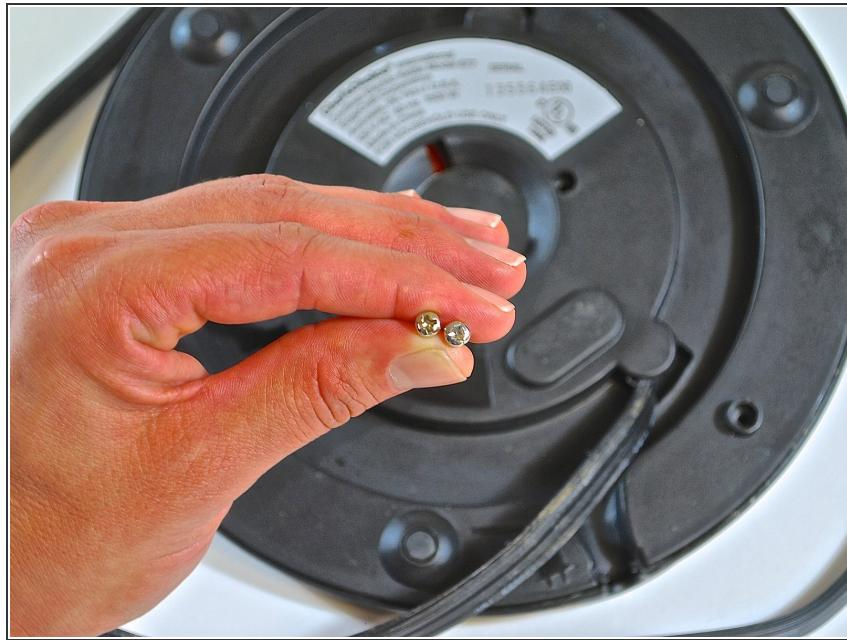
ⓘ There are two DIFFERENT kinds of screws on the base plate. • Three 3/8" standard Phillips screws • One 3/8" non-standard triangular Phillips screw. This image shows the difference between the two screws.
