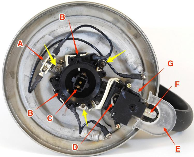
*(i)* Now that you have removed the bottom from the kettle, identify all of the parts. The YELLOW arrows point to the posts for mounting the control circuit components. The RED arrows point to the following parts:
