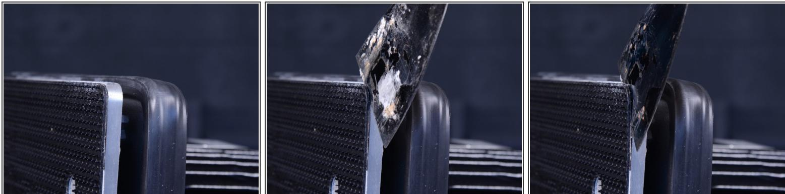
*(i)* The grip face pad is attached to the base plate by a layer of spongy adhesive.
