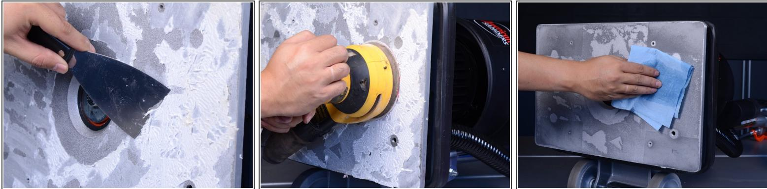
***i*** In order for the new grip face pad to adhere properly, you must remove all uneven adhesive residue from the base plate.
